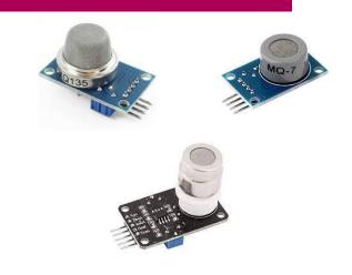
These sensors are calibrated based on the datasheet by finding the RS/R0 Ratio which is the main element for the measurement of gases by the gas sensors. At first these sensors are calibrated in fresh air and measured R0. Then these sensors are subjected to various gases and Rs is determined which is used for getting the ppm from the graph available in the datasheet.
