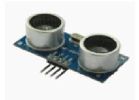
The Ultrasonic Sensor integrated with Arduino is used for sewage overflow detection. This will continuously monitor the sewage level so that the overflow can be prevented in advance.
